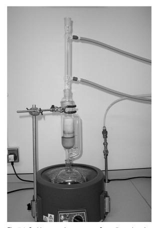
**Fig. 7.1** Soxhlet extraction apparatus. Generally used to give greatest yield of extract when extracts are stable in hot solvent.
