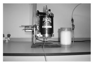
**Fig. 7.3** Biotage flash chromatograph. Fast separations are achieved with good resolution.
